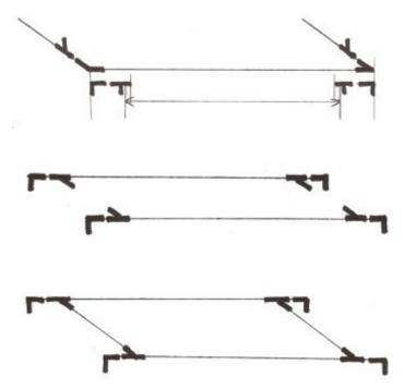
Place an elbow and a Tee touching each other along one end of the front of the base. Place another Tee and an elbow touching each other along the other end of the front of the base.
